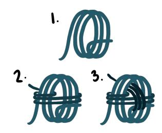
Make a Monkey Fist Knot on one end of the rope. Tighten the knot, and leave about 10-20cm at the end for a tongue.
